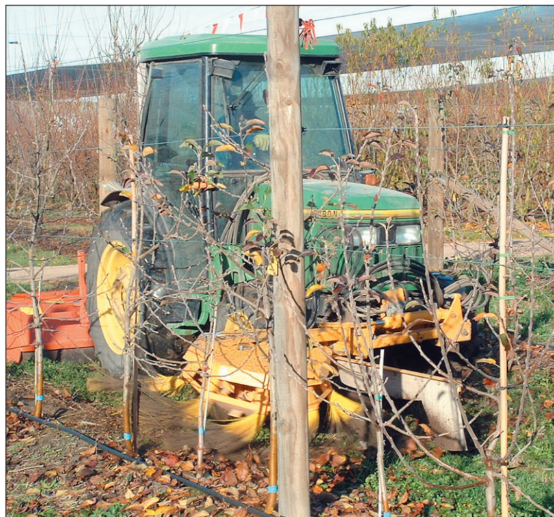
The Sadie leaf sweeper mounted on the front of a tractor. The rear-mounted flail mower mulches the leaves, thereby reducing over-wintering black spot and alternaria spores
