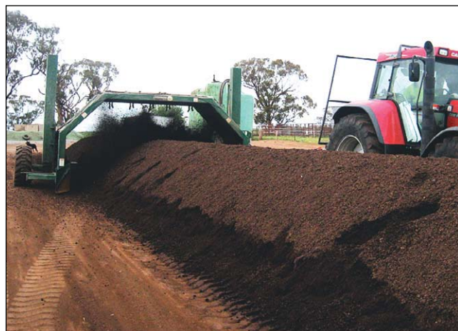
Aeromaster PT-170 Compost Turner on the YLAD Compost Site at Young NSW.
