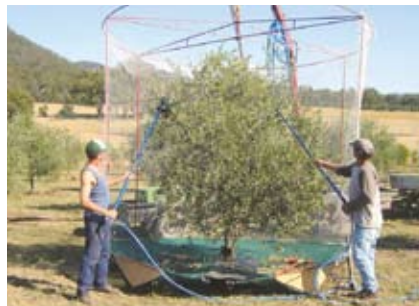
The Lakelands Catcher – an olive catcher designed by Lakelands Olives.
