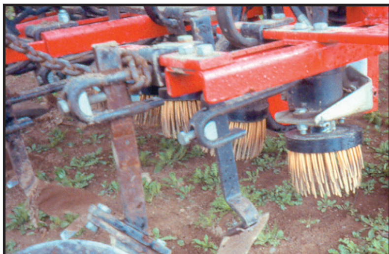
Vertical brushweeder, Sweden. Picture: Andrew Bishop, Tasmanian Department of Primary Industries, Water and Environment.
